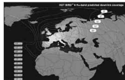
The Ku-band signal power level footprint for *Hot Bird-6*. Most of central Europe and S and SE England lie within the 53 dBW contour.
